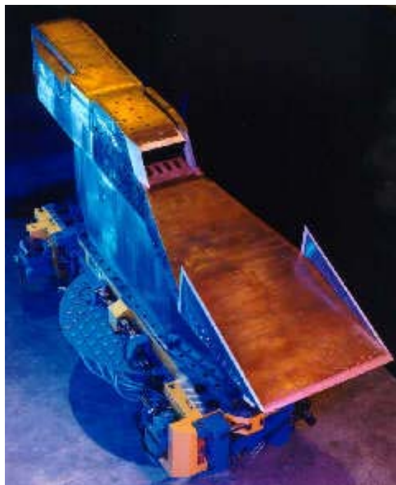
Figure 12 - 2-D engine model tested at Mach 6.8
