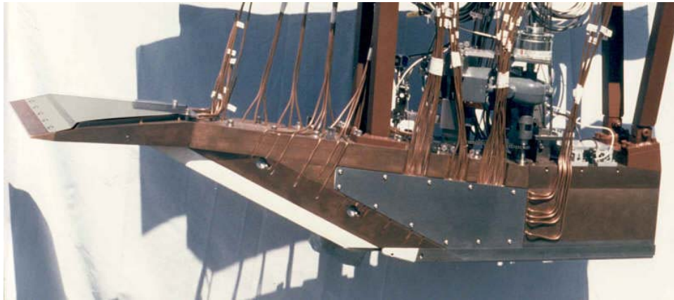
Figure 11 - 3-D Sidewall compression inlet model
